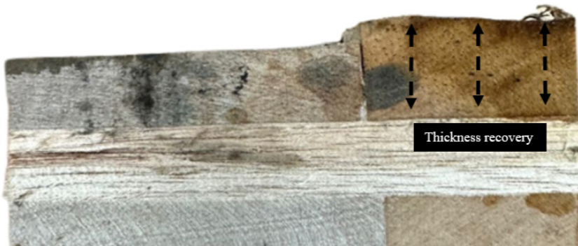
Fig. 8. Thickness recovery of the densified lamina layer upon prolonged exposure to fire.
