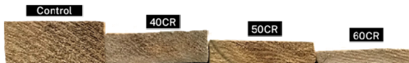
Fig. 2. Laminas pressed with different compression ratios (40%–60%).
