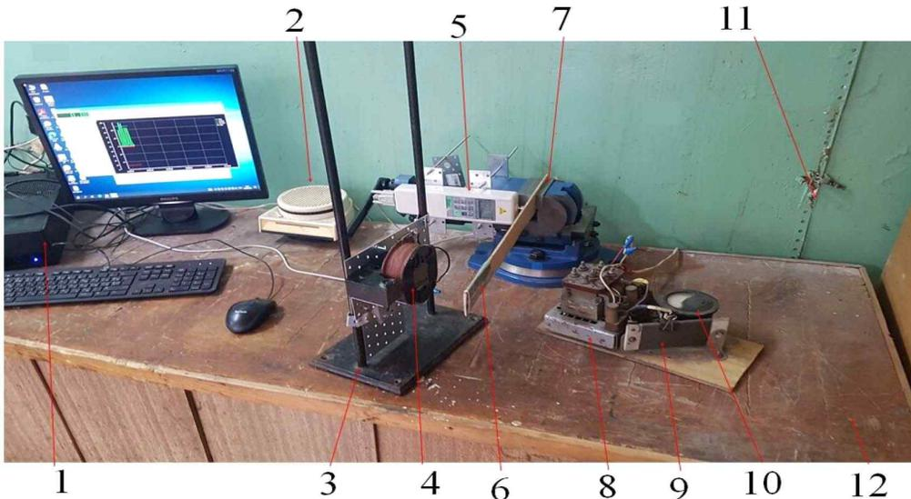
**Fig. 3.** Laboratory equipment. 1: computer, 2: stabilizer, 3: carrier, 4: magnet, 5: dynamometer, 6: sample, 7: three-position tool, 8: electro transformer, 9: electro corrector, 10: ampermeter, 11: protective tool, 12: digital desktop.
