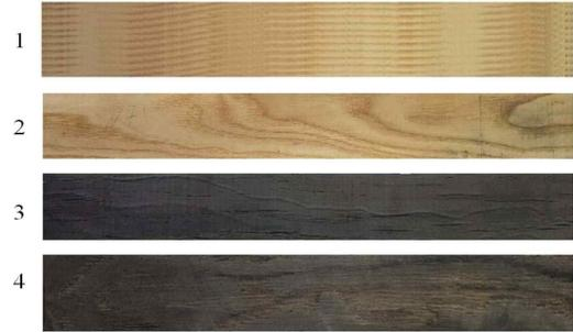
**Fig. 1.** Appearance of samples of the tested wood. 1, 2: oak natural, 3, 4: oak stained. The top-bottom or bottom-top direction corresponds to the 1: oak natural radial direction, 2: oak natural tangential direction, 3: oak stained radial direction, 4: oak stained tangential direction. Left-right is the lengthwise direction of the lumber, and the wood fibers are in the longitudinal direction.
