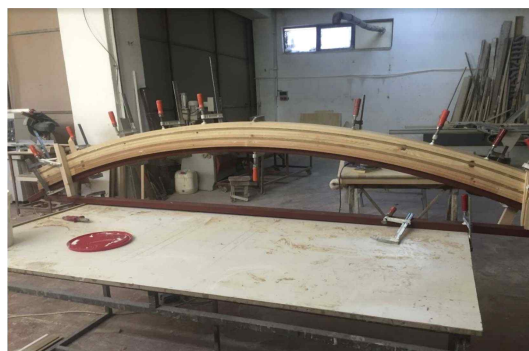
Fig. 1. Production phase of laminated systems in wooden structures.
