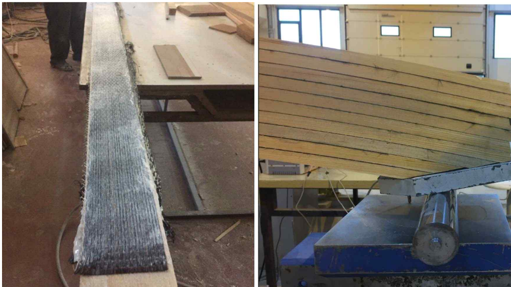
Fig. 3. Production stage (place of CFRP fabrics between layers). CFRP: carbon-fiber-reinforced polymer.
