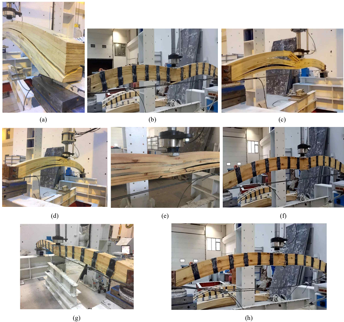
Fig. 12. Crack pattern and failure modes of reference timber arches. (a) (R) Laminated wood, (b) RF specimen, (c) 3F specimen, (d) 5F specimen, (e) 7F specimen, (f) 3FF specimen, (g) 5FF specimen, (h) 7FF specimen.
