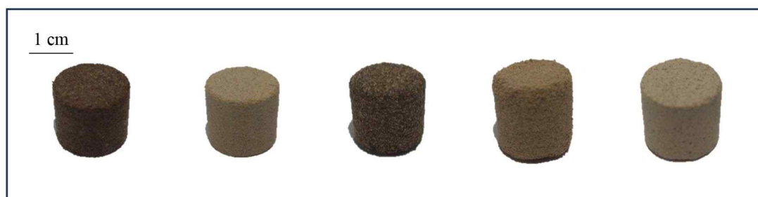
Fig. 1. Produced biopellets. From left to right: Lagerstroemia speciosa , Ganophyllum falcatum , Myrsine avisin , Mischoecarpus sundaicus , and Gigantochloa atter .
