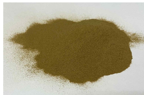
Fig. 7. Sorted chopped woody greenery (fraction < 0.2 mm).
