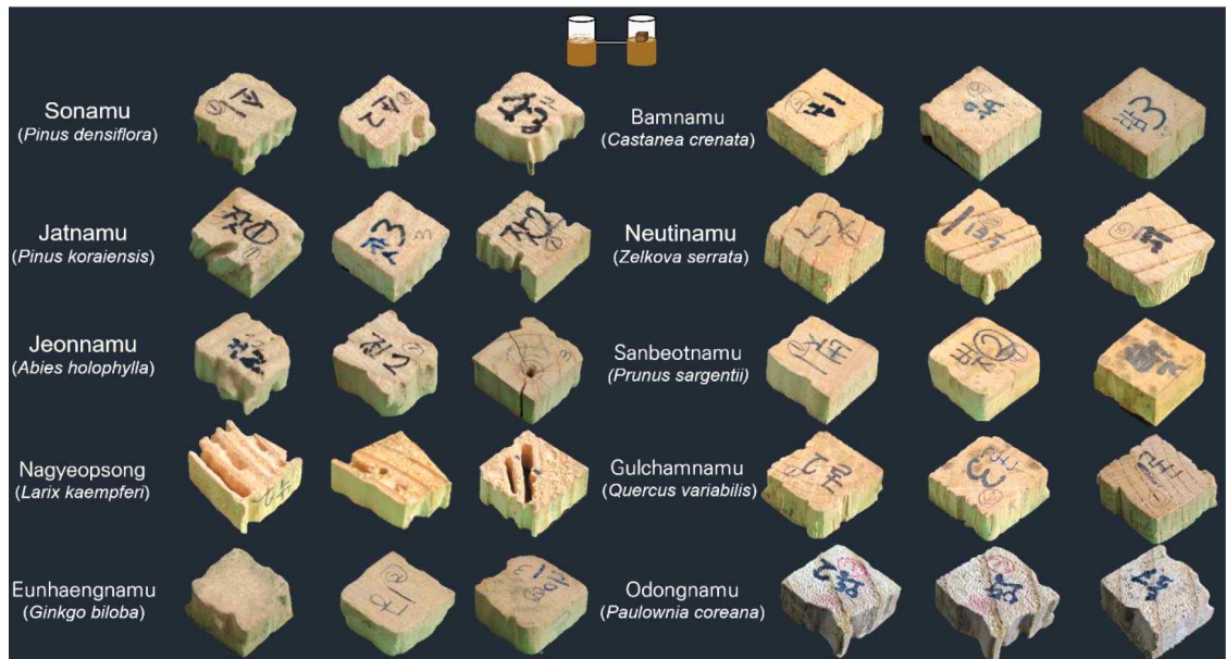
Fig. 2. Wood damage caused by Reticulitermes speratus in the no-choice test.
