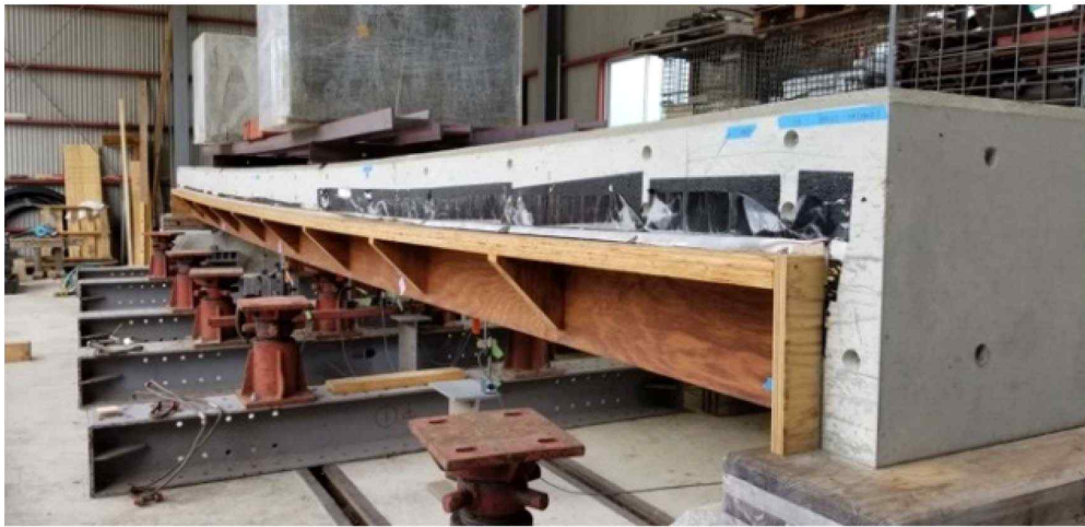
Fig. 1. Test LVL specimen. LVL: laminated veneer lumber.
