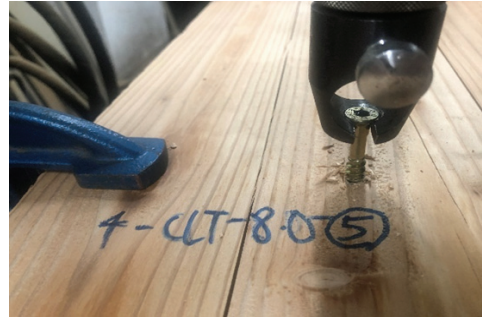
Fig. 3. Failure mode of specimen.
