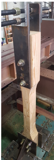
Fig. 4. Photograph of tensile strength test.
