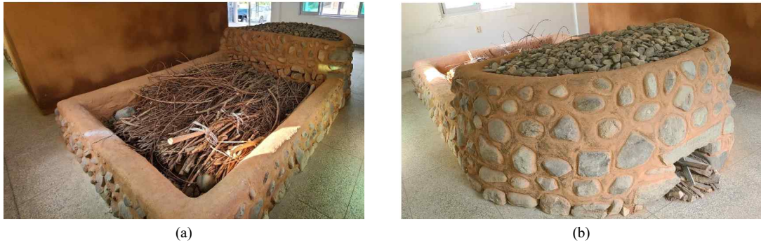
Fig. 1. A traditional Daknamu steaming facility for traditional Hanji making, recreated in the exhibition hall located in the Demonstration Culture Village in Bongsu-myeon, Uiryong-gun, Korea. (a) A room for a pile of Daknamu shoots, (b) a space for a stone pile and fire.
