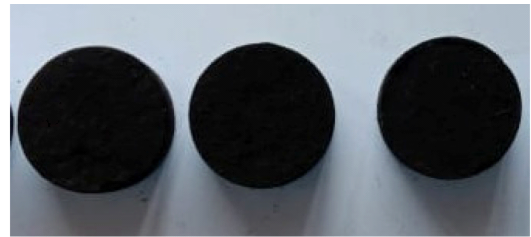
Fig. 5. API briquettes. API: added pine resin.
